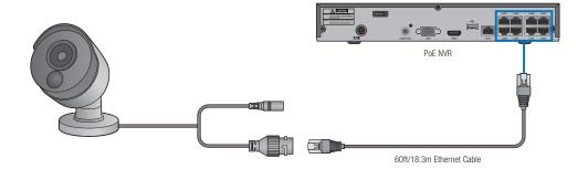
Note: The power connector is provided as an alternative power option if required. Your NVR will provide power over the Ethernet cable when connected and a separate power adapter is not required.
